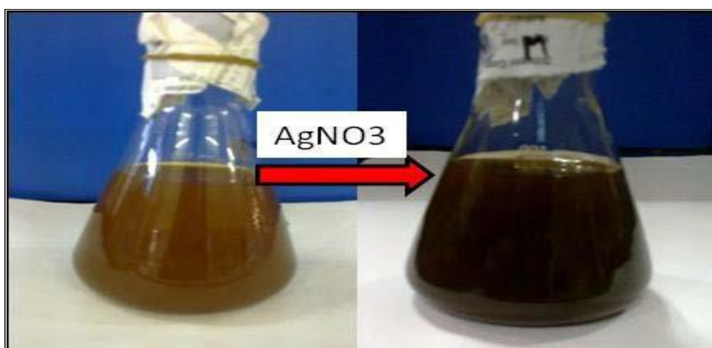
Fig 1 : Colour change of plant extract before and after addition of AgNO 3
